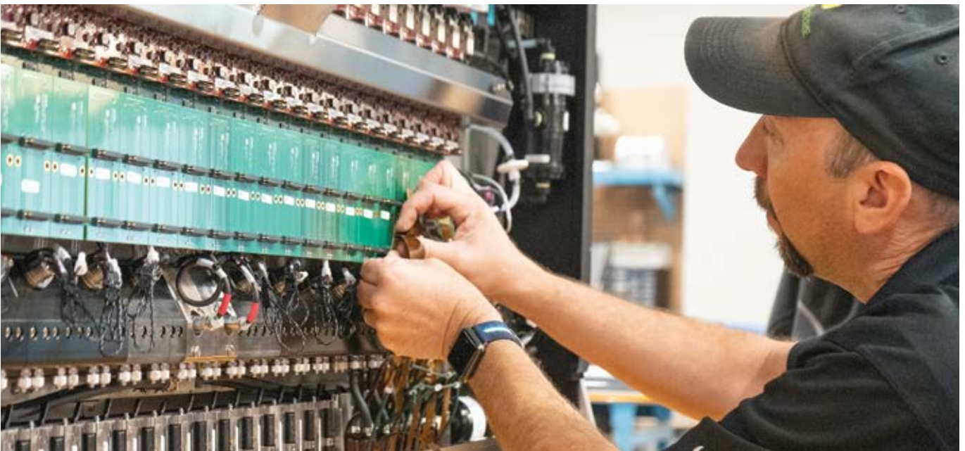
A 40-inch (1016mm) Fujifilm 42K print bar system under construction
